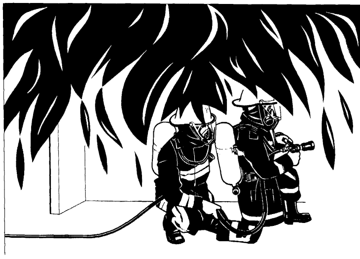
Figure 2 A delayed backdraught
