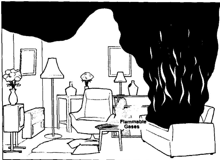
Figure 4 The build up of the smoke layer
