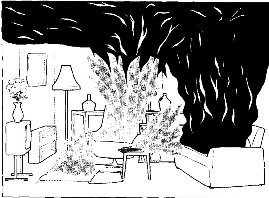
Figure 6 Rapid heating of all combustible materials
